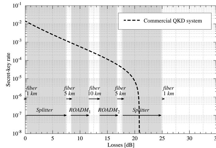
The figure compares 1) the secret key rate of a commercial QKD device with 2) the losses experienced traversing the different components of a metropolitan optical network.
