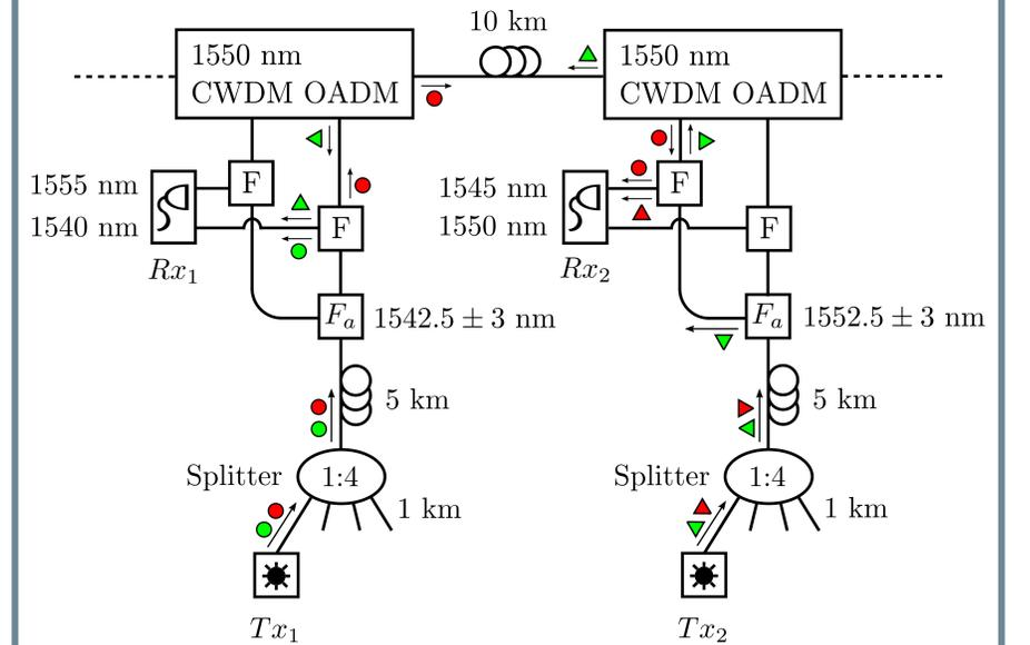
Communications between emitters and receivers are represented using colored circles (from  $Tx_1$ ) and triangles (from  $Tx_2$ ). The color indicates the wavelength. There are two different paths joining  $Tx_1$  with  $Tx_2$ , e.g. via  $Rx_1$  or  $Rx_2$ .
