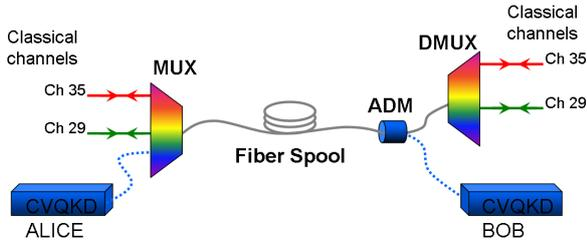
Figure 2: Experimental setup. Each classical channel is used to test noise from forward and backward transmission.
