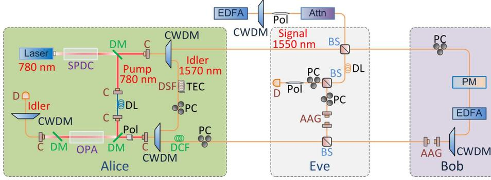
Figure 1: Experimental setup. SPDC: spontaneous parametric downconverter; DM: dichroic mirror; C: collimator; CWDM: coarse wavelength-division multiplexer; BS: beam splitter; Attn: attenuator; EDFA: erbium-doped fiber amplifier; DL: delay line; PC: polarization controller; PM: phase modulator; AAG: adjustable air gap; Pol: polarizer; DCF: dispersion-compensating fiber; DSF: dispersion-shifted fiber; TEC: thermoelectric cooler; OPA: optical parametric amplifier; D: detector.
